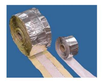
**Composition - Information on Ingredients:** Metallic 3 inch wide adhesive Aluminium tape with an acrylic adhesive, covered with siliconized paper, with 1 inch strip of continuous filament glass fiber tape running down the centre. Fibrous glass (E-type, continuous filament); Composition consisting of oxides of silicon, aluminium, calcium. boron and magnesium, fused in an amorphous vitreous state.
