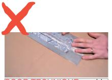
POOR TECHNIQUE would be to just stick tape down - as this allows air to be traped.
